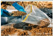
Fill the sample bag with a wellmixed, composite sample.
