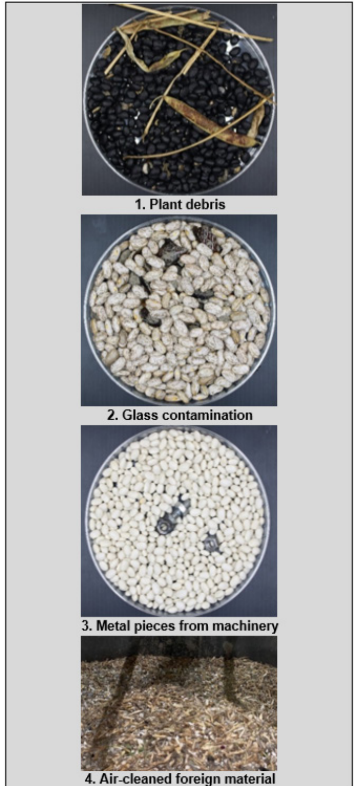
Image 9: Unacceptable presence of foreign materials including plant debris (1), glass from roadsides (2), metal from equipment failure (3) foreign material removed by air aspiration during receiving at point of delivery (4). Source: Original images by Evan Wright and Michigan Bean Commission.
