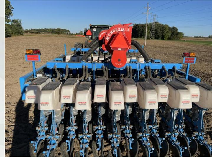
**Ongoing research:** New custom-build planter with capacity to plant in 5" row spacing (using 2 toolbars, with row units spaced 10" apart on each)
